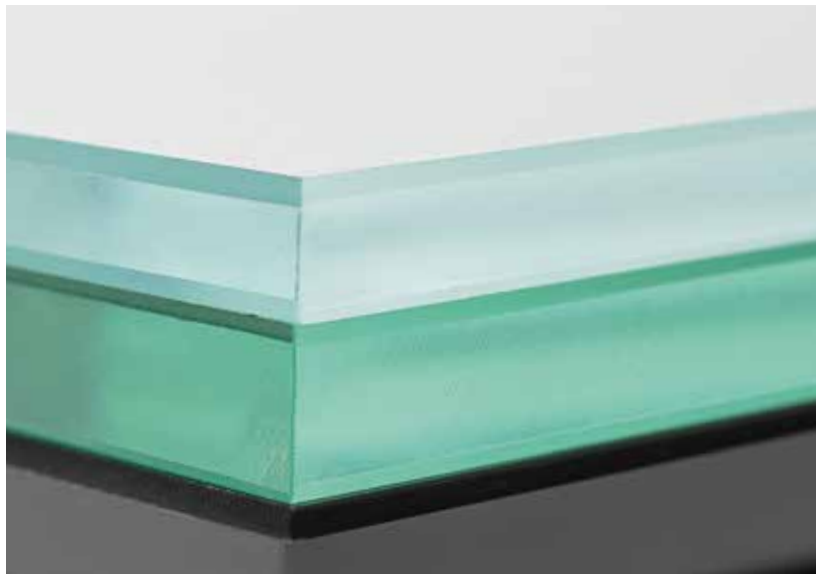
The difference between normal float glass and low-iron glass
