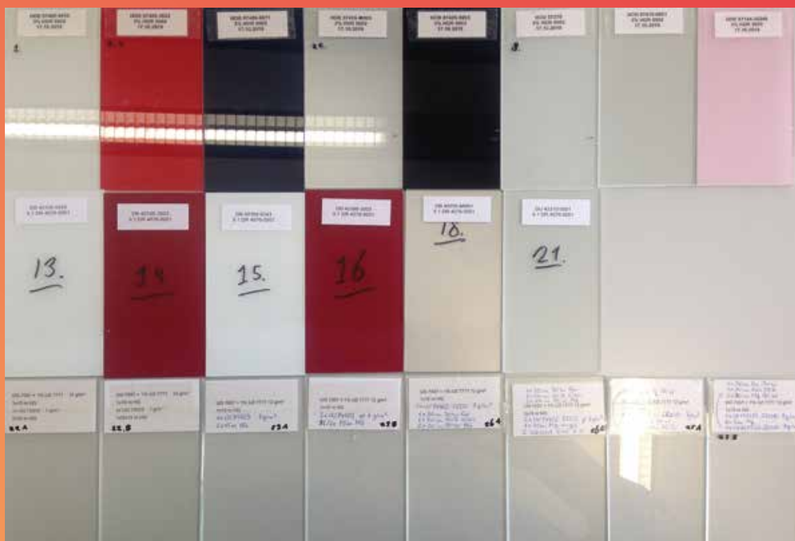
QUV test surfaces (*) for testing resistance to UV radiation from sunlight
